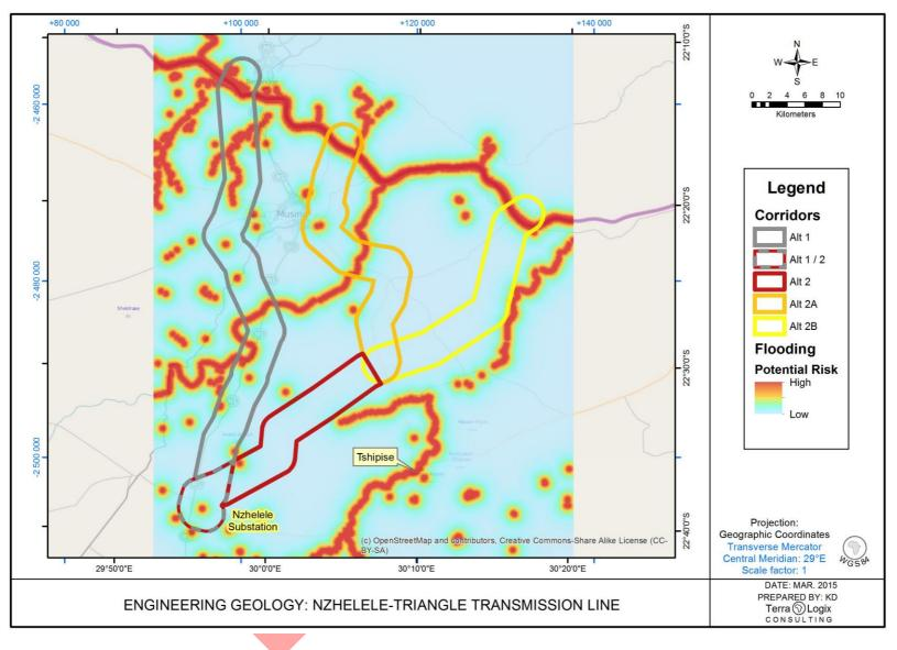
Figure 6 Potential risk due to flooding
