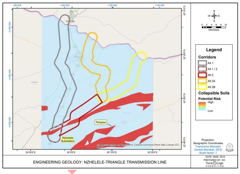
Figure 9 Potential risk due to collapsible soils
